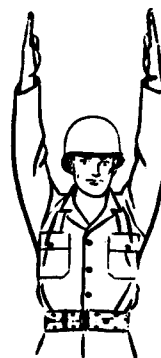
This way, this marshaller, desired landing direction, or desired landing point. (Pilot will make his approach toward the marshaller's front.) Hold arms rigid and overhead, palms facing inward (STANAG 3117).
